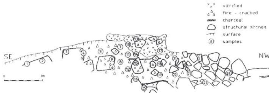
Fig. 3. Section through the vitrified rampart of Broborg, showing sample locations (in circles).
